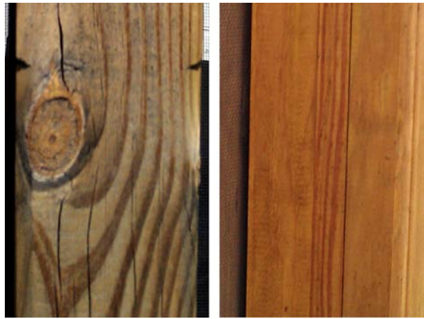
Solid Post #2 Grade with splits and knots (left) vs. 3x laminated post clear grade no split no knots
